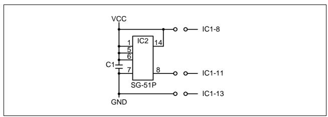
Figure 2 Connection diagram when using the C1
